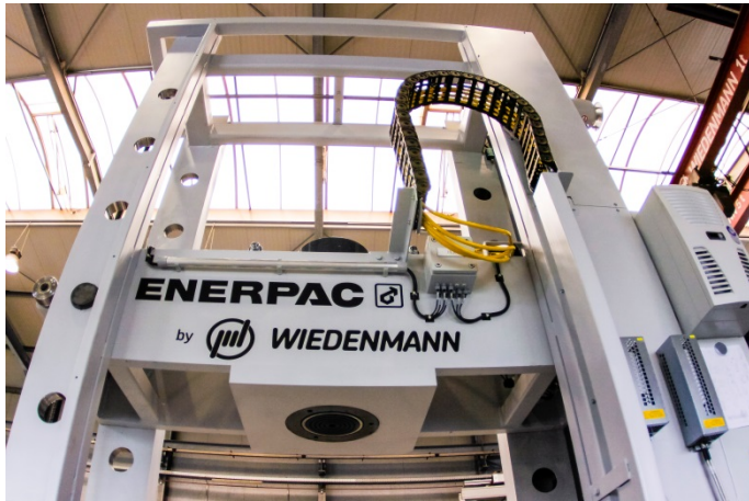
Picture 6: The electronically adjustable upper yoke can be set in five stages of 400 millimetres via a spindle drive and operating panel.
