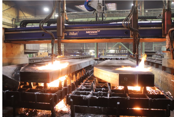
Picture 12: The profiling was performed with several burners operating in parallel.
