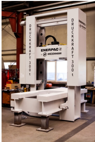
Picture 3+4: For this four metre high and 2.8 metre wide roll frame press with 3,193 kN (300 tonnes) of pressing force, a table length of 3.8 metres and 13 tonnes tare weight, Jebens welded press table and base components of the upper yoke.
