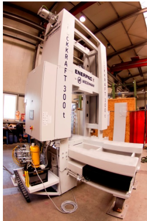
Picture 3+4: For this four metre high and 2.8 metre wide roll frame press with 3,193 kN (300 tonnes) of pressing force, a table length of 3.8 metres and 13 tonnes tare weight, Jebens welded press table and base components of the upper yoke.
