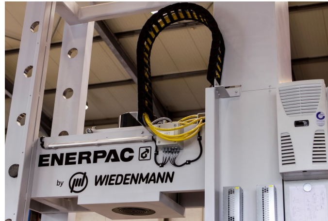
Picture 5: The massive welded and completely electrified roll frame construction is movable along a distance of 1,750 millimetres.
