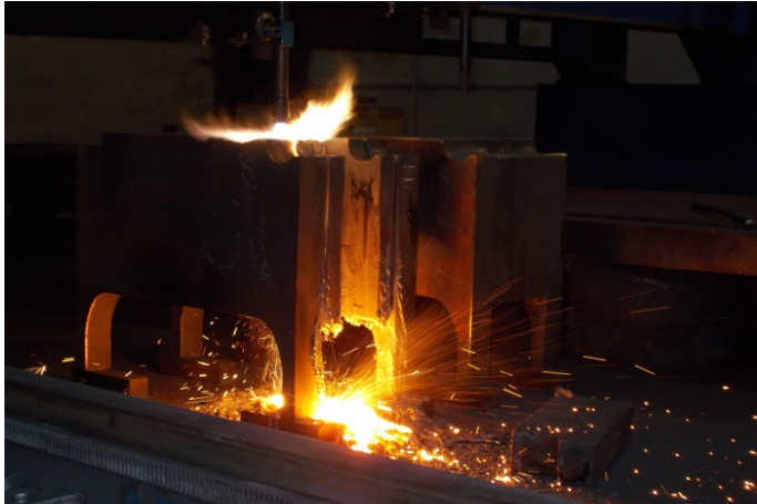
Picture 11: The fine-grained steel was pre-heated to 150 degrees Celsius and parameters such as oxygen pressure and the cutting speed were set accordingly.
