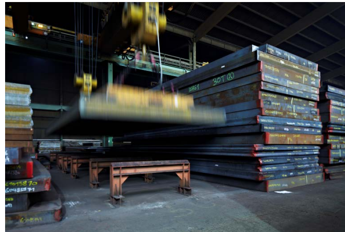
Picture 10: The availability of high-strength steels in their own stock - in thicknesses from 30 to 300 millimetres – spoke in favour of Jebens.
