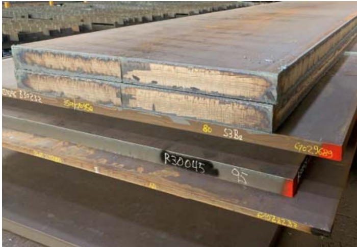
Picture 1: High-speed order for Jebens: two plates – each measuring 7,700 mm long, 1,900 mm wide and 150 mm thick with flame cuts for maritime salvage.
