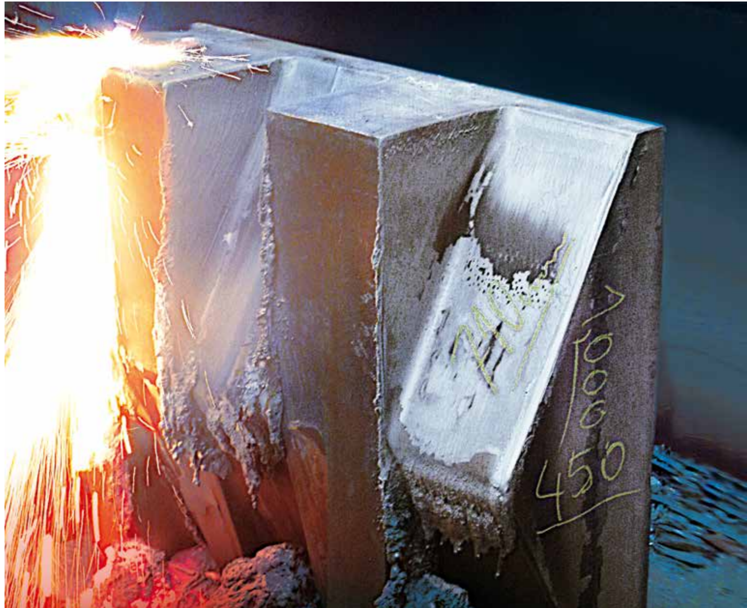
2.3 Technology FLAME CUTTING Application: Spare part for a steel mill Steelgrade: S355JR+AR Weight / Dimensions: 6,318 kg / 450 x 1,300 x 1,350 mm Particularity: Extreme chamfer with a length of 710 mm
