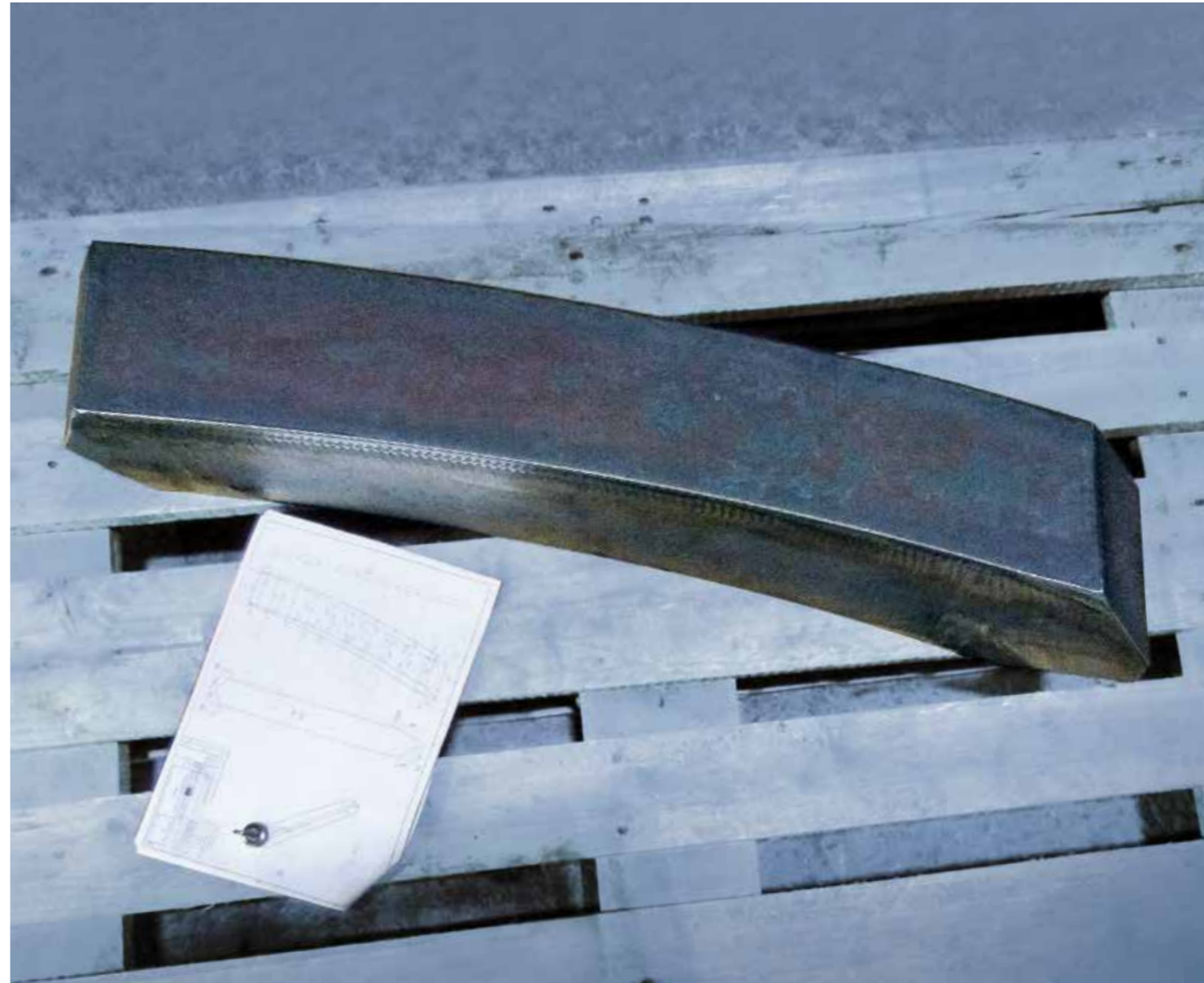
2.4 Technology FLAME CUTTING Application: Spare part of a steel converter Steelgrade: P355NH Weight / Dimensions: 218 kg per piece / 120 x 245 x 928 mm Particularity: The chamfering angle is changing constantly over the total length of the piece
